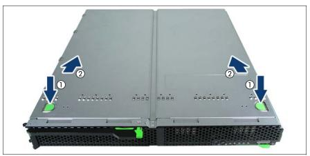
Figure 9: Removing the cover
